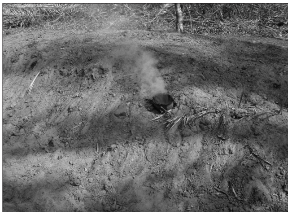
Figure 9.5 Production of biochar using simple earthen mound kilns
